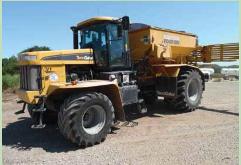
*Skyland Grain LLC has a six-bin truck for variable-rate application. This gives us the ability to apply up to six products exactly where they are needed based on grid sampling—all in one pass through the field.*
